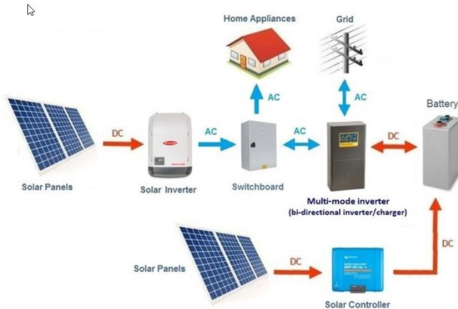
Combination AC and DC Coupled system - Can be configured as Grid-interactive or Off-grid with generator
