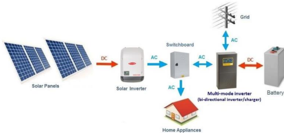
Basic layout diagram of an AC coupled solar battery system - Grid-tie (hybrid) setup
